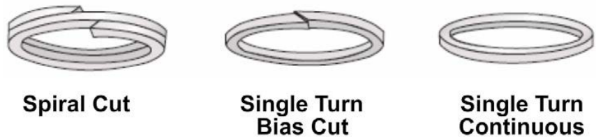
Figure 7-15 — Types of backup rings.
